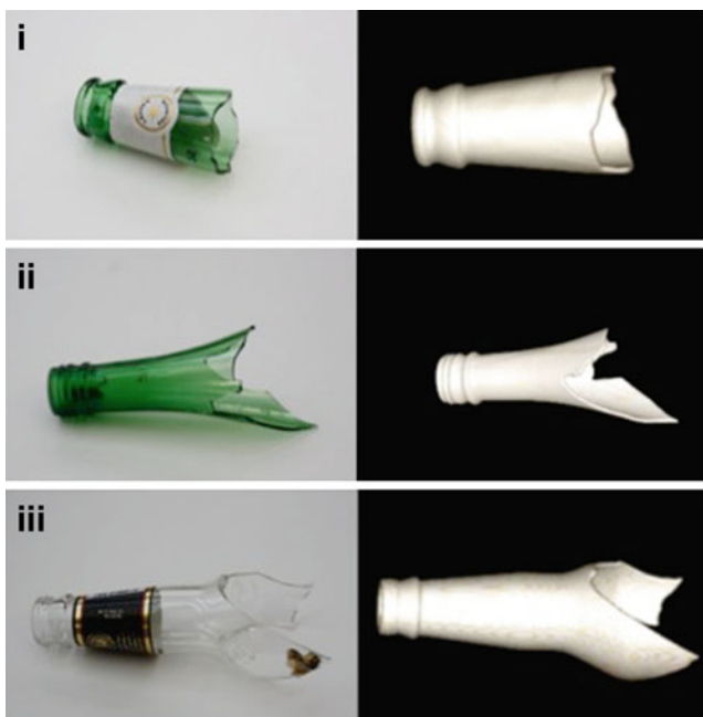
Fig. 2 Typical fracture patterns that were observed are shown (both as an image and an MDCT image) (1) tulip, (2) bayonet and (3) extended shards
